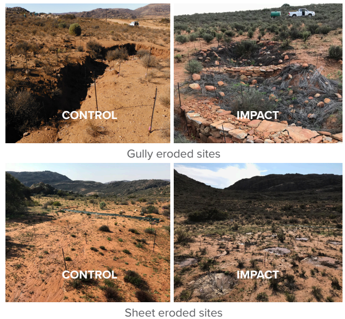
Figure 3 | Placement of erosion pegs as part of the Before-After-Control-Impact-Paired (BACIP) design on sheet (bottom) and gully (top) eroded sites, where interventions were placed on Impact (right) but not Control (left) sites).
