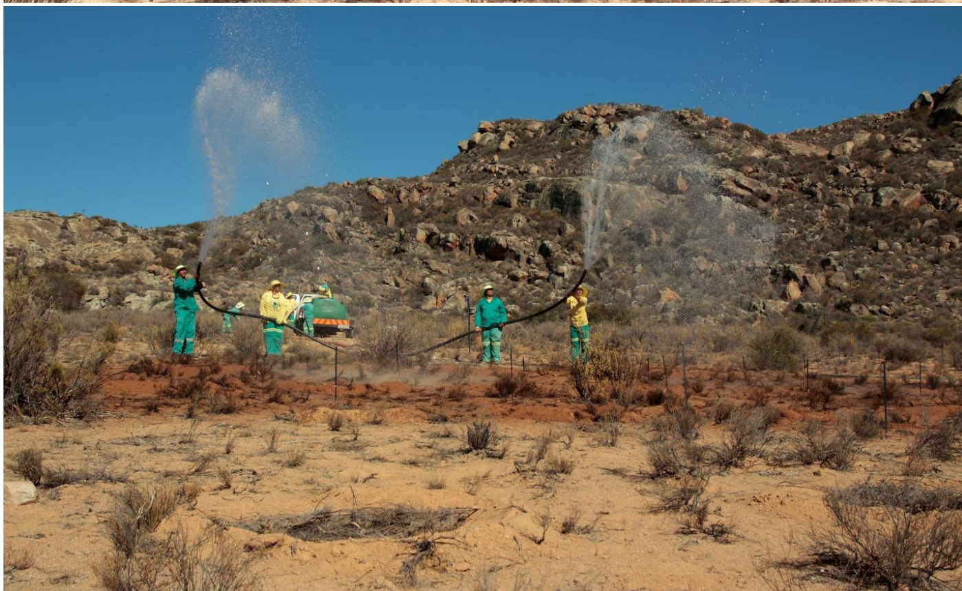
Figure 4 | Rainfall simulation and infiltration experiment using a series of water pipes connected to spray heads (top), which received water from a water bowser via a petrol pump and sprayed over the paired sites until run-off occurred (bottom).
